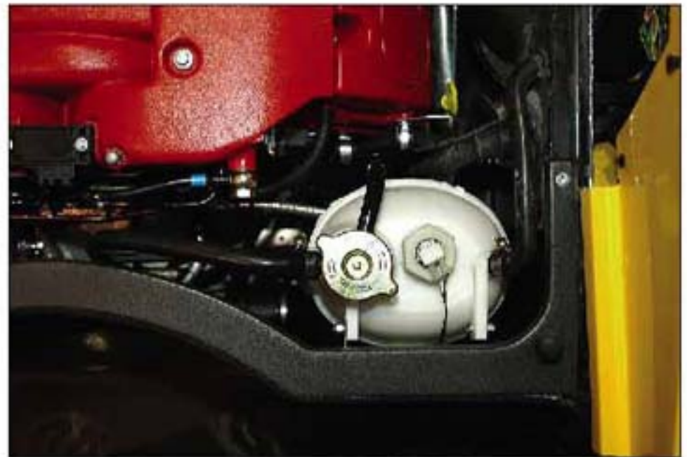
020 ABOVE VIEW OF COOLANT HEADER TANK
