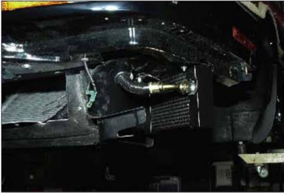
009 VIEW OF LH OIL COOLER
