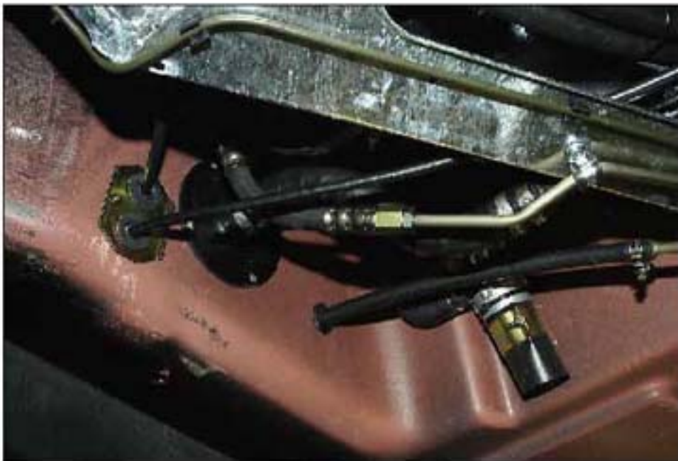
011 VIEW OF ENGINE COOLING RECIRCULATING PUMP
