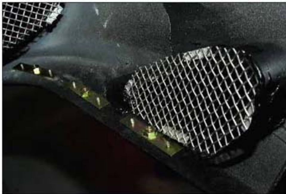
007 REVERSE VIEW OF AIR INTAKE GRILLES
