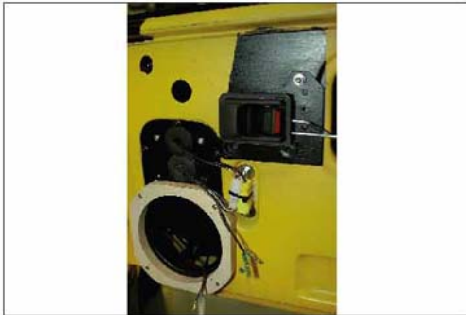
007 VIEW OF DOOR LATCH & RADIO SPEAKER INSTALLATION
