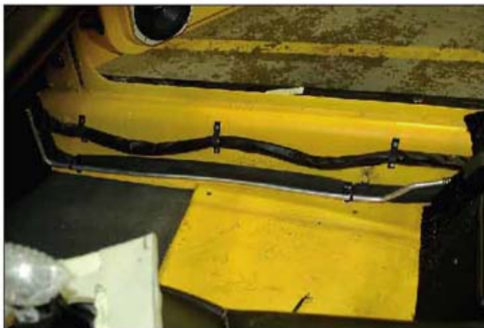
005 LH SIDE VIEW OF WIRING LOOM ROUTING
