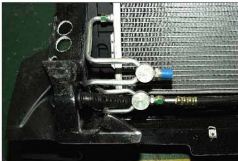
005 AC CONDENSER SUB ASSEMBLY
