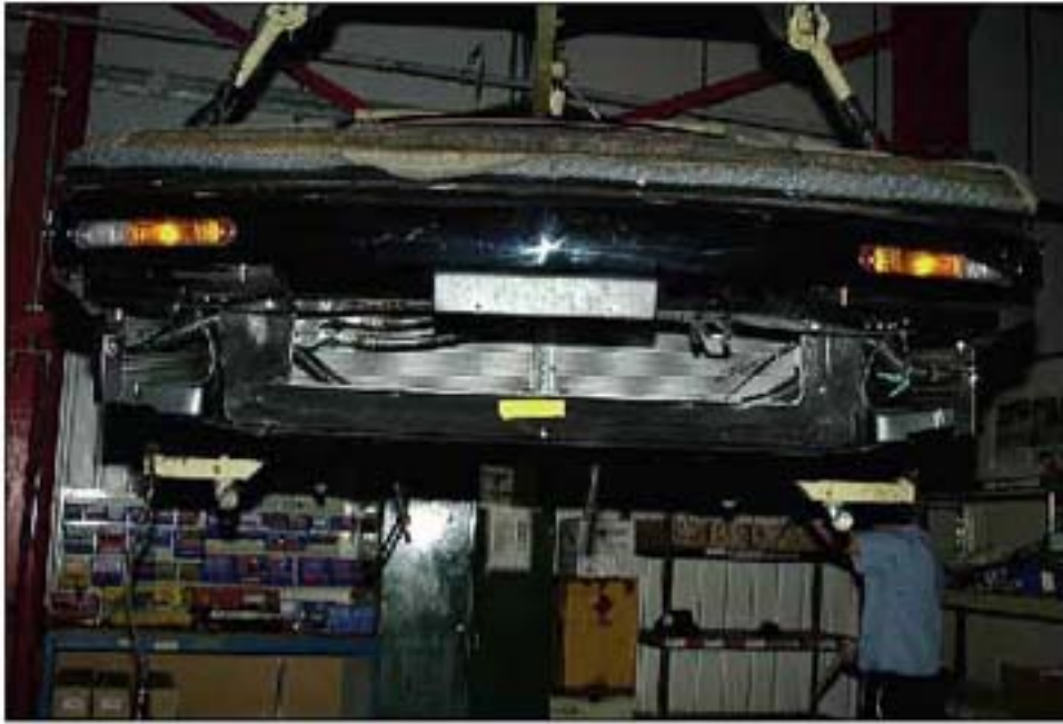
007 FRONT VIEW OF COOLING SUB ASSEMBLY IN SITU
