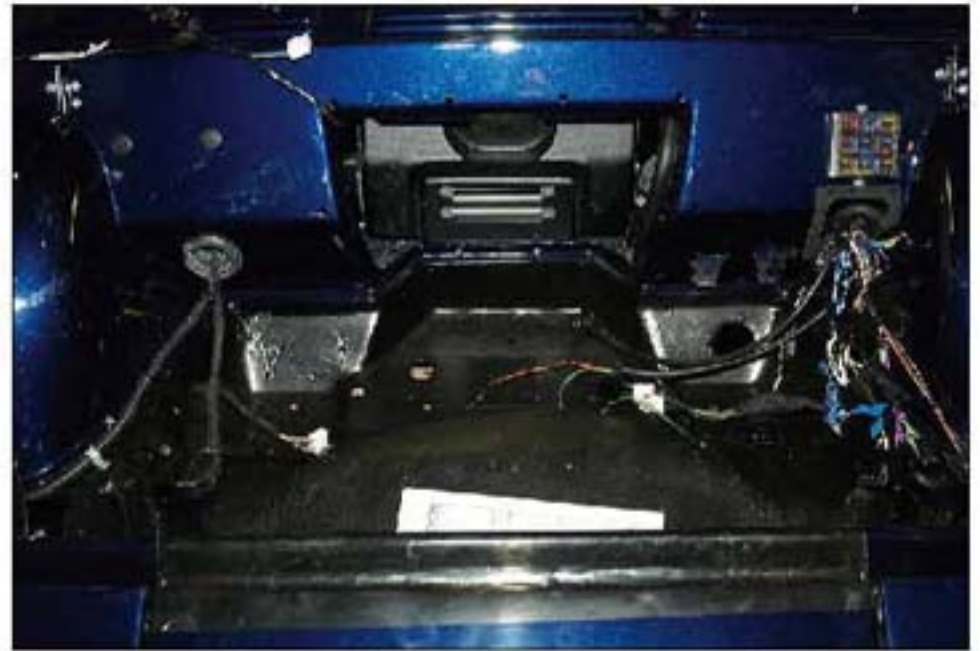
001 FRONT VIEW OF HEATER APERTURE
