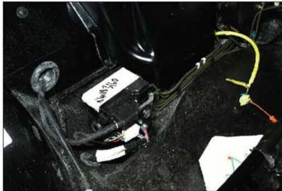
003 FRONT VIEW OF ABS MODULE
