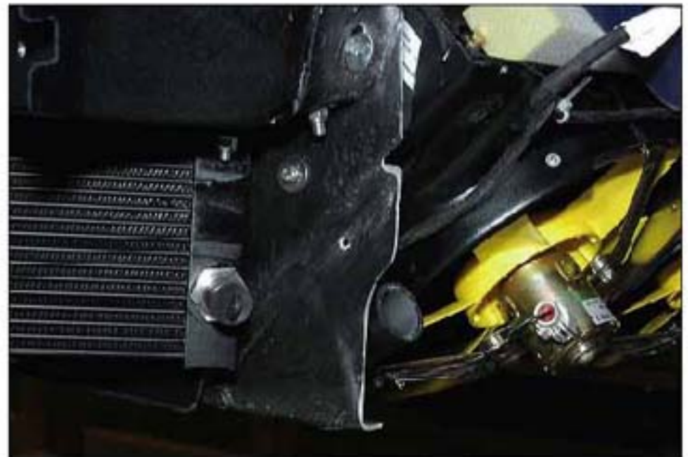
012 LH SIDE VIEW OF LH OIL COOLER
