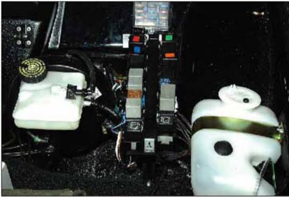
007 FRONT VIEW OF RELAYS
