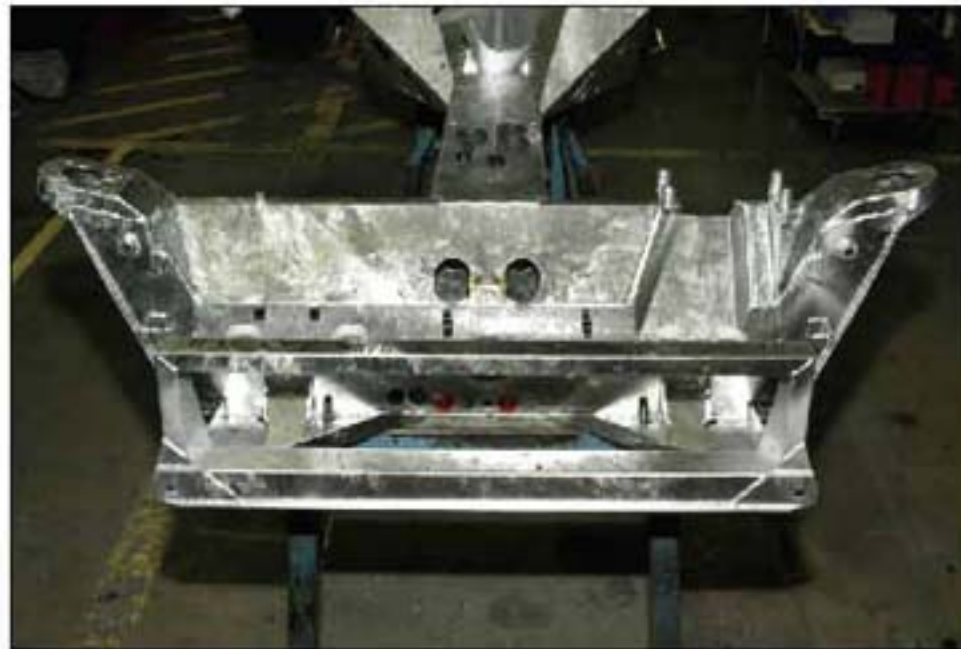
003 VIEW OF CHASSIS FRONT SECTION
