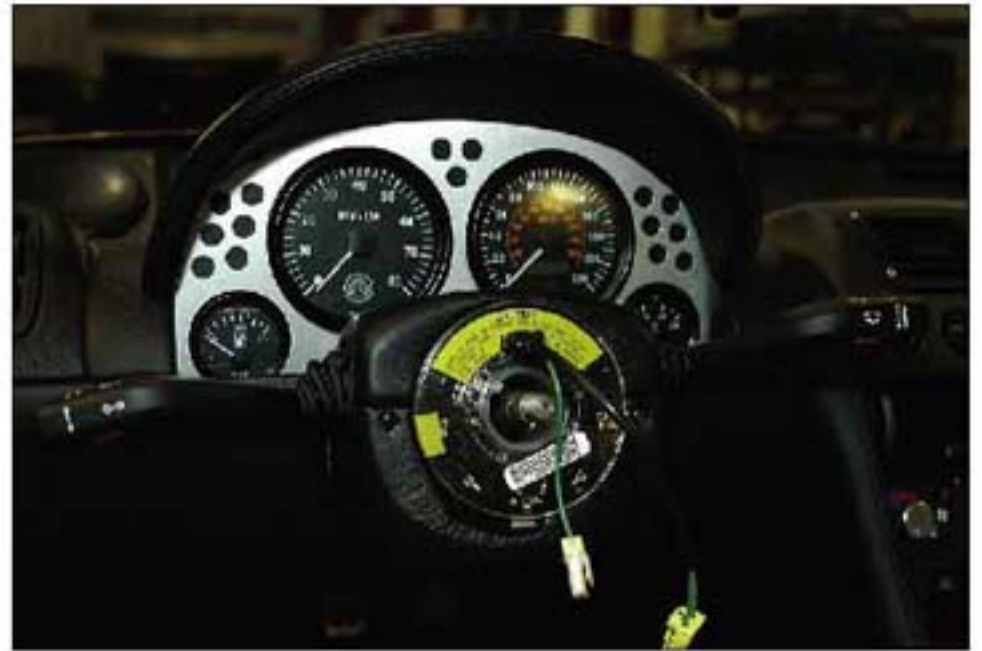
001 VIEW OF INSTRUMENTS & PETRI COIL
