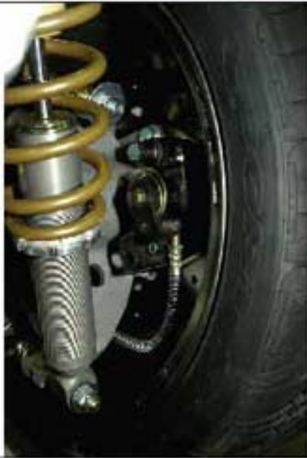
023 REAR OBLIQUE VIEW OF RH REAR BRAKE CALIPER
