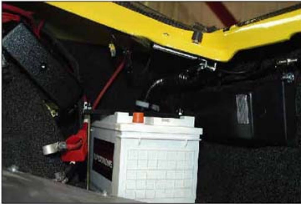
017 VIEW OF BATTERY IN STOWAGE AREA
