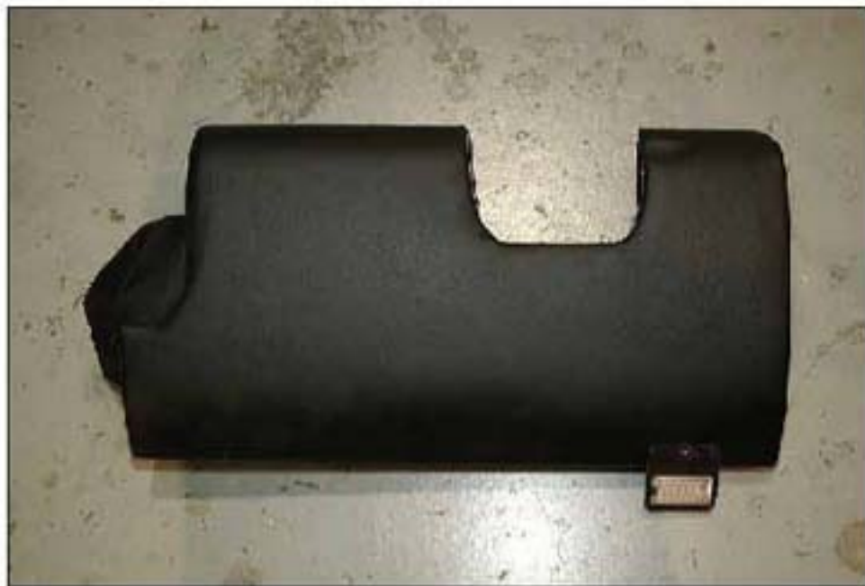
026 FRONT VIEW OF DRIVER'S KNEE BOLSTER
