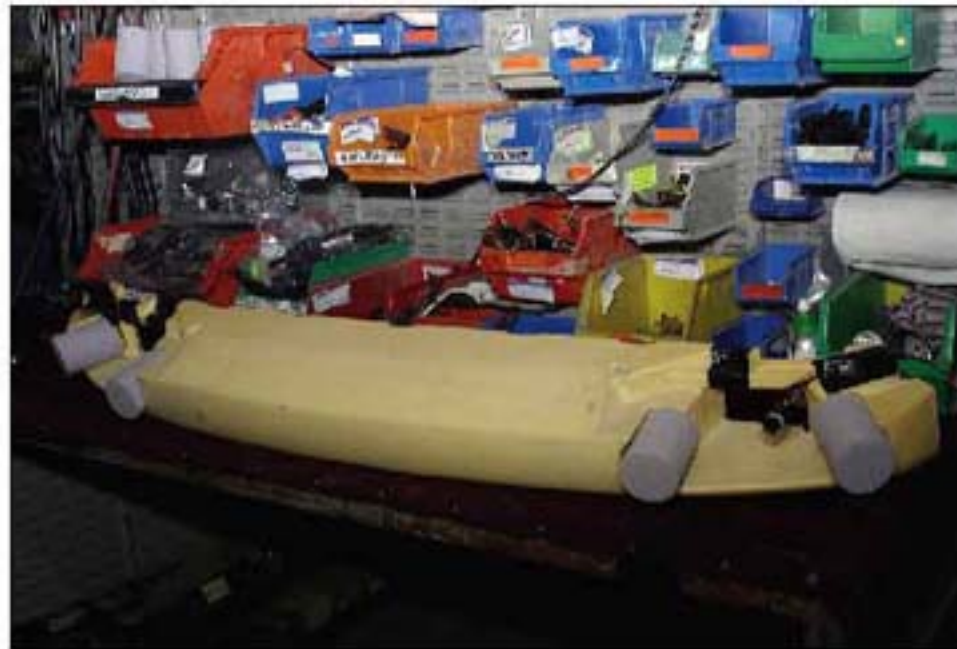
003 FRONT BUMPER CRASH ARMATURE
