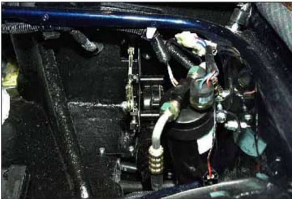
013 VIEW OF RECEIVER DRYER
