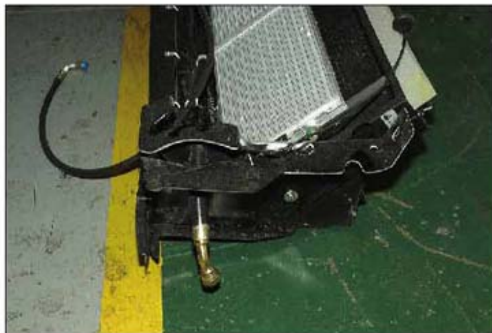
006 AC CONDENSER SUB ASSEMBLY
