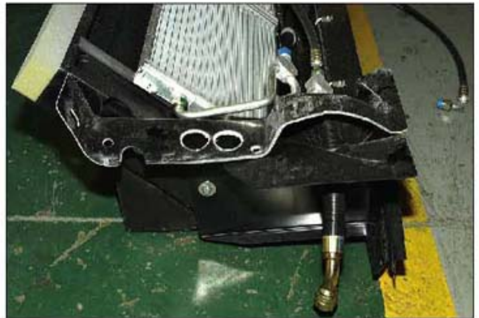
004 AC CONDENSER SUB ASSEMBLY
