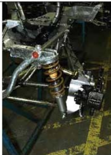
021 REAR VIEW OF RH REAR SUSPENSION
