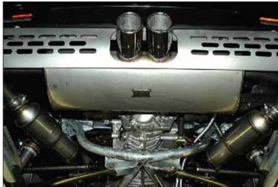
003 REAR VIEW OF EXHAUST MUFFLER/CATALYST
