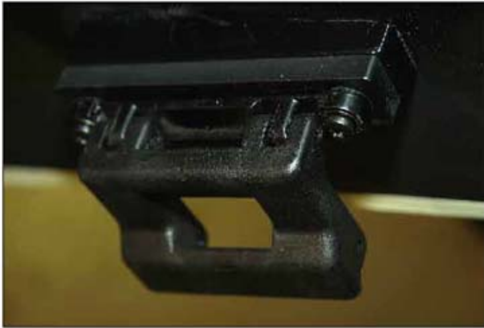
017 VIEW OF ROOF PANEL RELEASE CATCH
