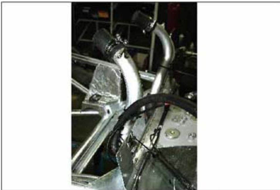
011 RH SIDE VIEW OF ENG COOLING PIPES
