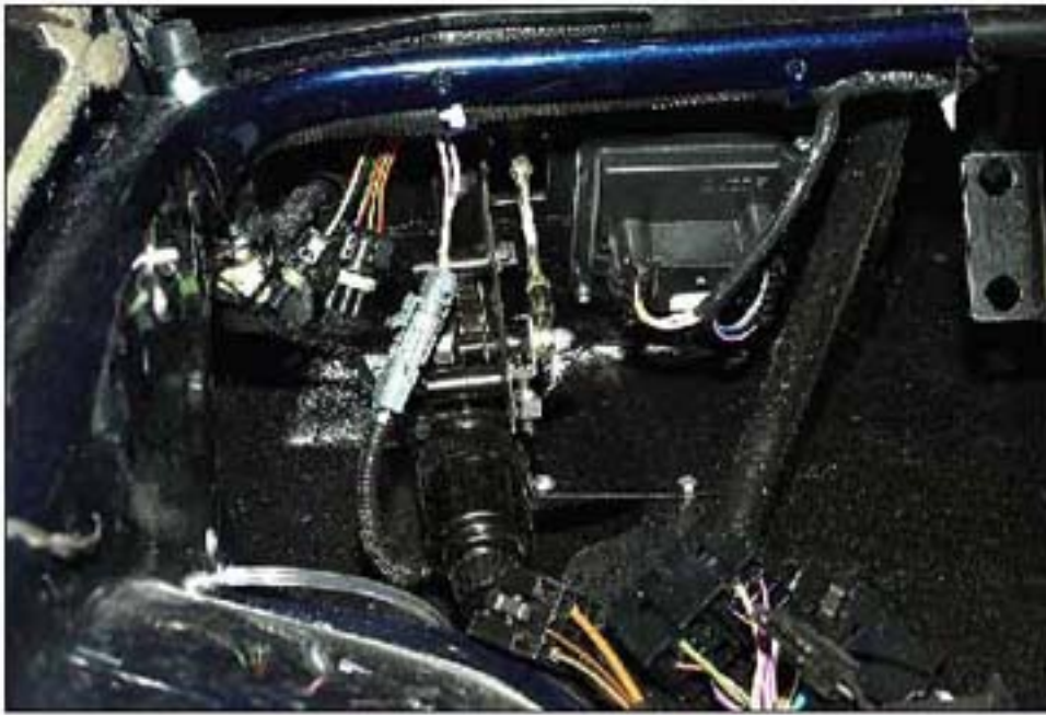
009 REAR VIEW OF LH HEADLAMP LIFT MOTOR
