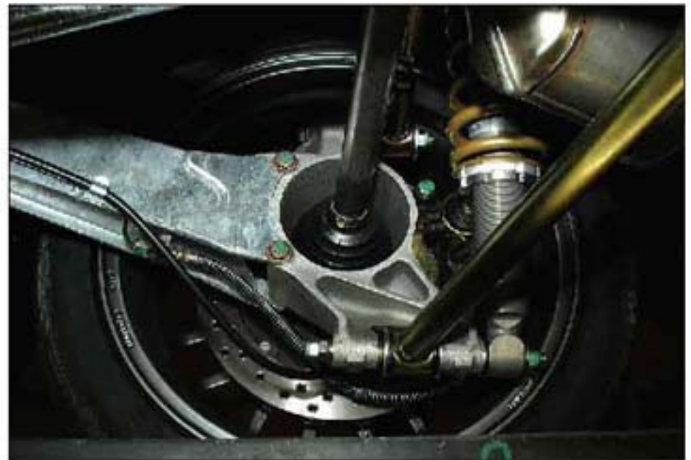
014 VIEW OF RH REAR HUB ASSEMBLY
