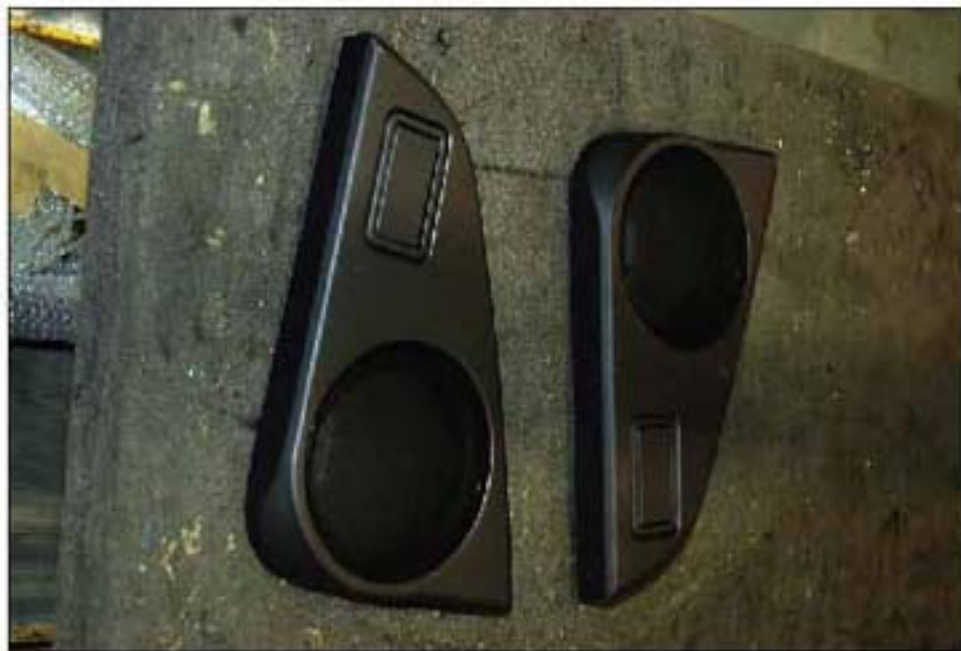
010 FRONT VIEW OF DOOR SPEAKER PANELS
