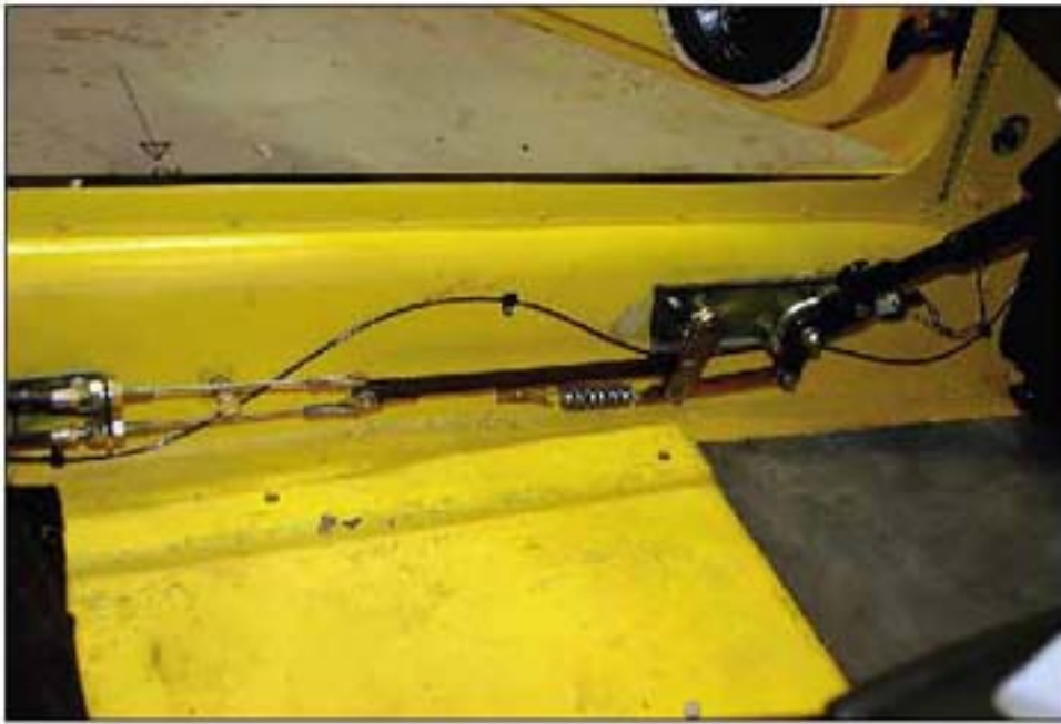
007 RH SIDE VIEW OF HANDBRAKE INSTALLATION
