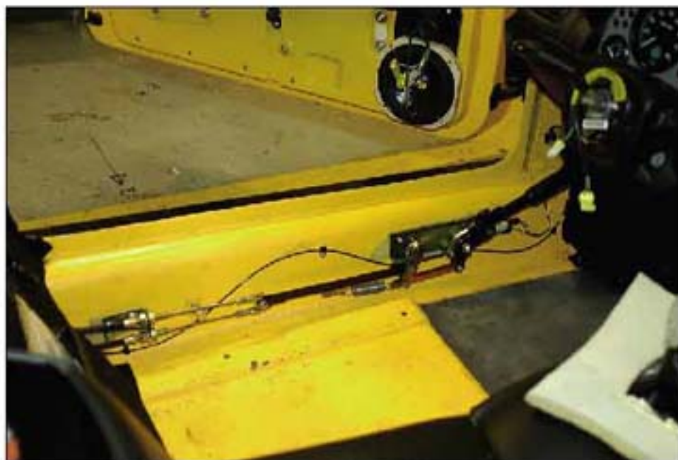
006 RH SIDE VIEW OF HANDBRAKE INSTALLATION
