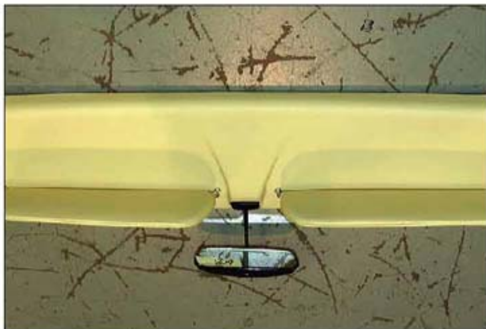
014 FRONT VIEW OF FRONT HEADER TRIM
