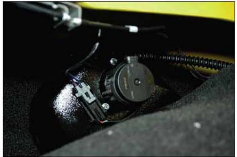
018 VIEW OF EMISSION AIR PUMP
