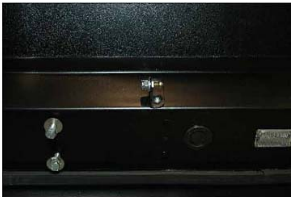
011 VIEW OF GAS STRUT PIVOT
