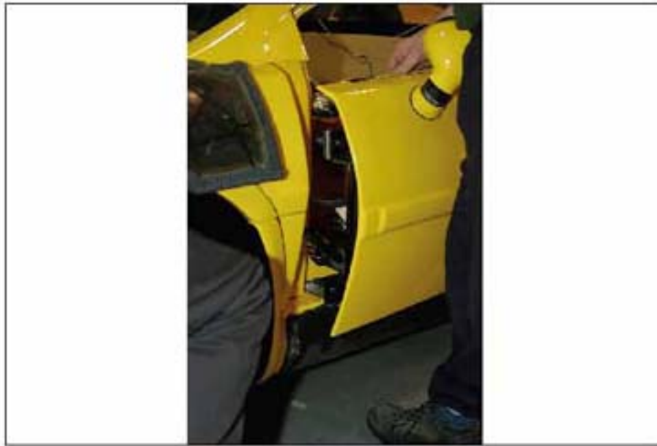
009 VIEW OF LH DOOR FITTING OPERATION
