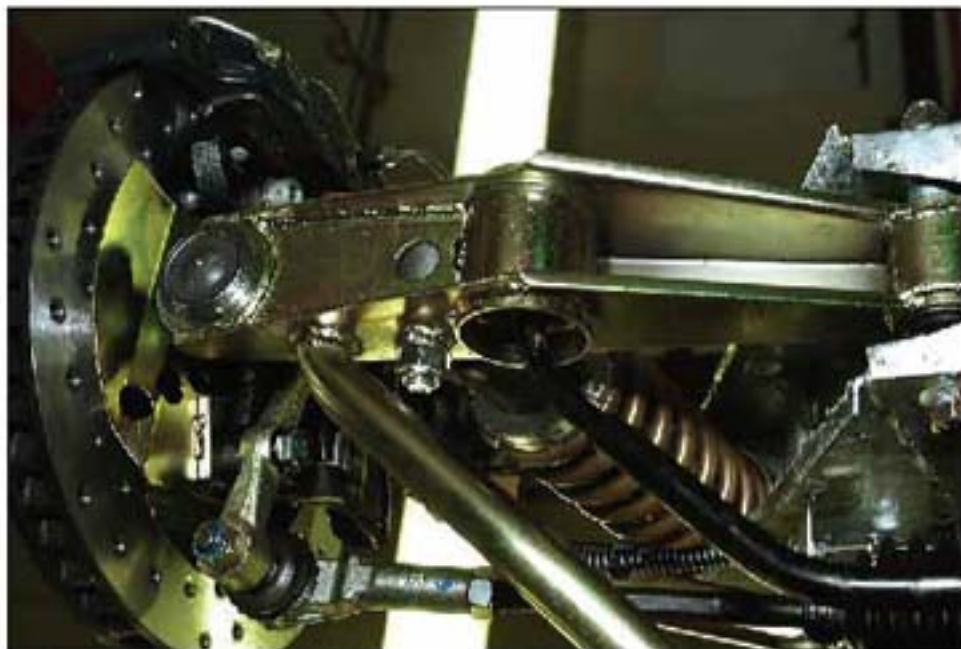
045 UNDERSIDE VIEW OF LH FRONT TRACK CONTROL ARM
