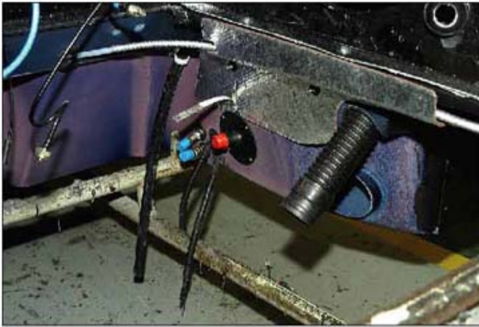
009 LH REAR OBLIQUE VIEW OF RH SIDE OF BODY ENGINE BAY
