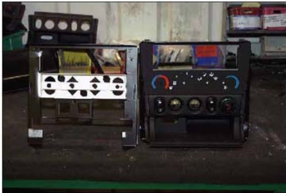
007 AC & HEATER SWITCH PANEL
