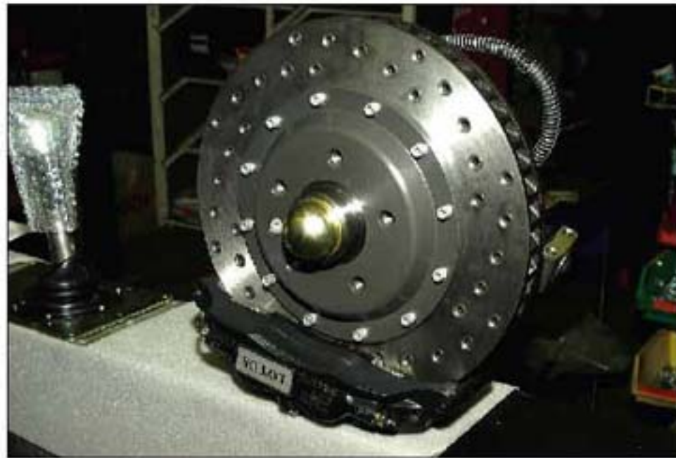
003 VIEW OF FRONT BRAKE SUB ASSEMBLY
