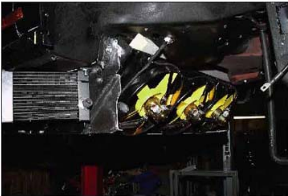
011 LH SIDE VIEW OF COOLING FANS
