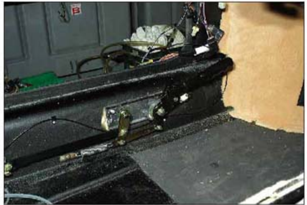
018 RH SIDE VIEW OF HAND BRAKE
