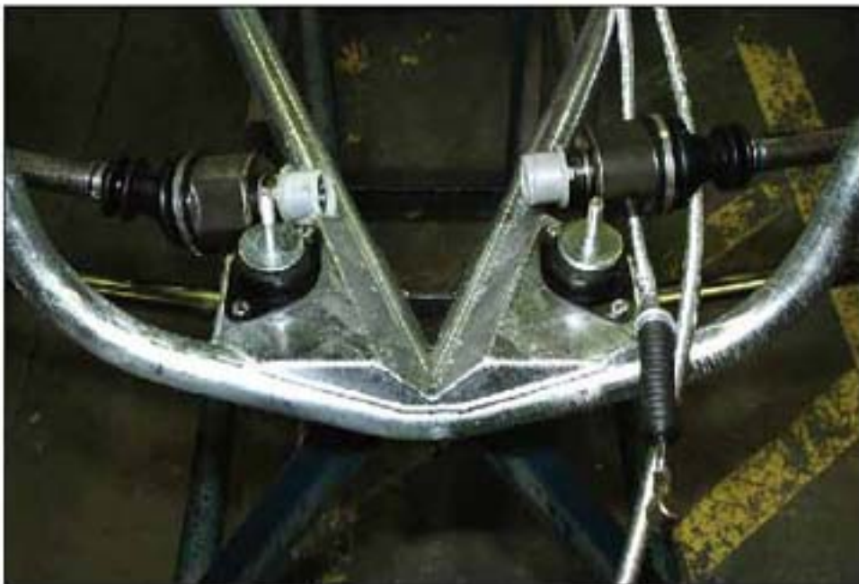
011 VIEW OF CHASSIS TRANSMISSION MOUNTINGS
