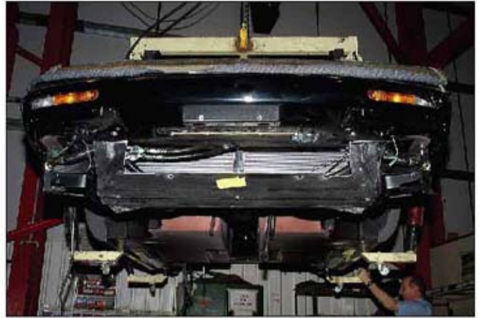
008 FRONT VIEW OF COOLING SUB ASSEMBLY IN SITU
