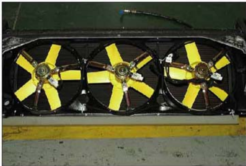
002 VIEW OF RADIATOR COOLING FANS
