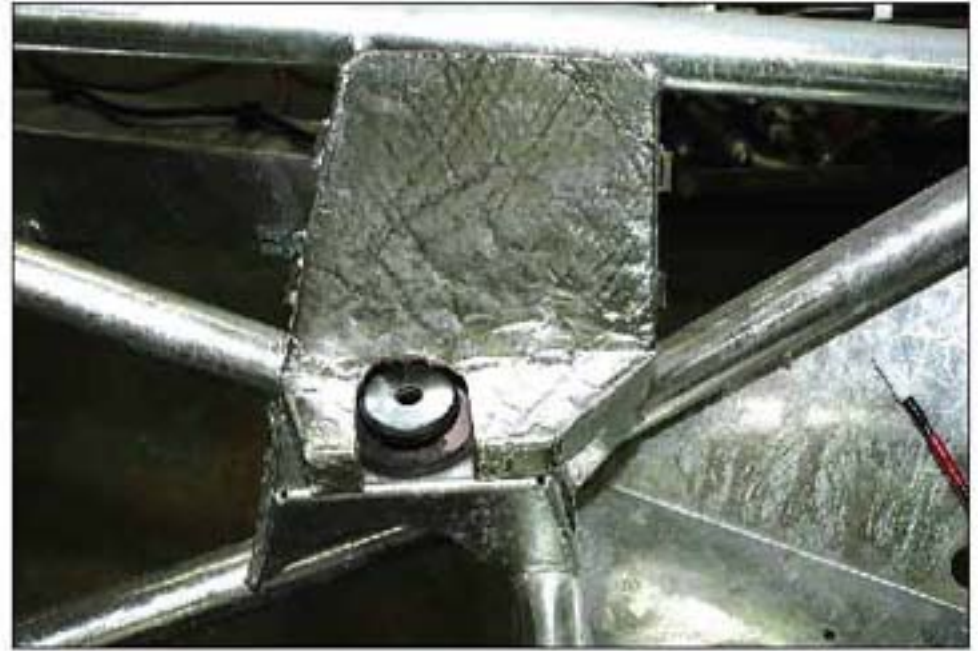
010 RH SIDE VIEW OF LH ENG MOUNTING
