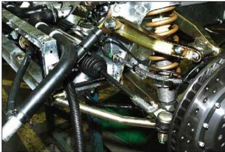
041 FRONT OBLIQUE VIEW OF LH FRONT SUSPENSION
