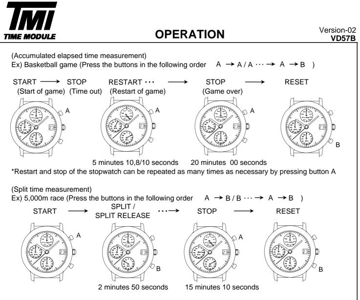
\* Measurement and release of the split time can be repeated as many times as necessary by pressing button B.
