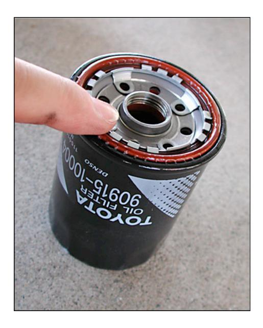
Lubricate the oil filter seal, the red ring around the opening. This will allow the seal to seat correctly on the mounting block. Note this <u>filter</u> is what Lotus is supplying in the Lotus labled box, as seen several pictures above.
