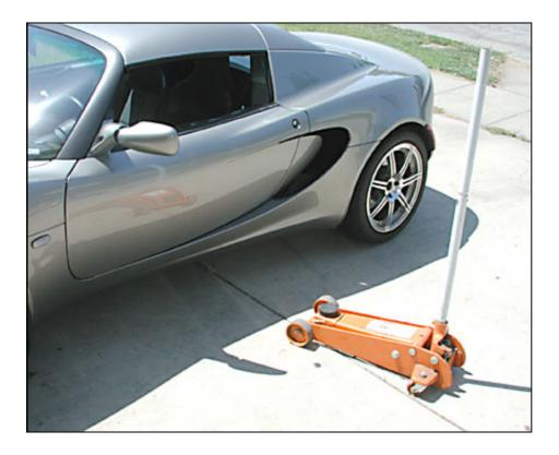
The jack is ready to be placed under the car. Notice the saddle, the part that touches the underneath part of the car, has a rubber disc on it. This is to distribute the load and not dent the bottom of the car. Use of a wide saddle, with an
