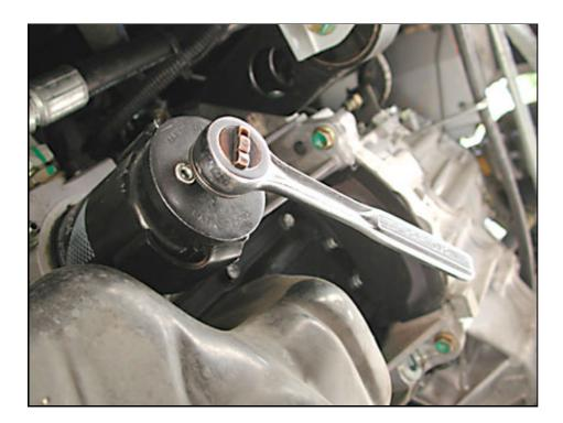
Here the oil filter is about to be removed. It unscrews just like a bolt. Watch out as more oil will drain from the sides of the top of the filter as you loosen it. Wait for it to slow and then remove the filter by unscrewing more. Please dispose of your oil and filter in such a way as not to harm the environment.
