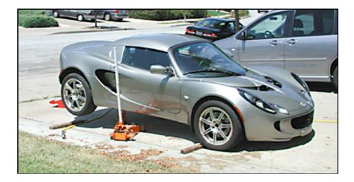
Place the jack on the other side of the car, raise the car the same way you did the first side, and place a second jack stand. Shake the car vigorously and make sure it is stable. It is better to fall off the stands now while you are not under it, than to fall later when you are working under it. My kids think I am a safety nut and they are right.
