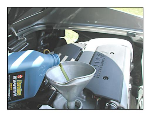
The oil fill cap is on the left side of the engine cover. I place a rag to catch any oil that spills from the bottle and pour with the opening on top, as shown. If you look closely, you will see a symbol embossed in the next of the container showing the same method. This prevents the oil from bubbling out and splashing around.
