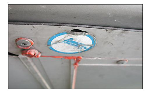
Examine the bottom of the car and look for the blue and white lift sticker. It has the symbol of a jack on it. Place the rubber disc under this sticker and start lifting the car.
