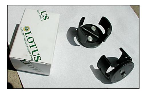
It helps to be very strong and have a massive grip when it comes time to remove the old filter I am neither. I purchased an oil filter removal tool at the local auto parts store. I recommend one that has a thick metal base, where your socket wrench attaches in the small square hole. Thin metal will bend, deform or even round off. The picture above contains two views of the tool and only one is needed to remove the filter.
