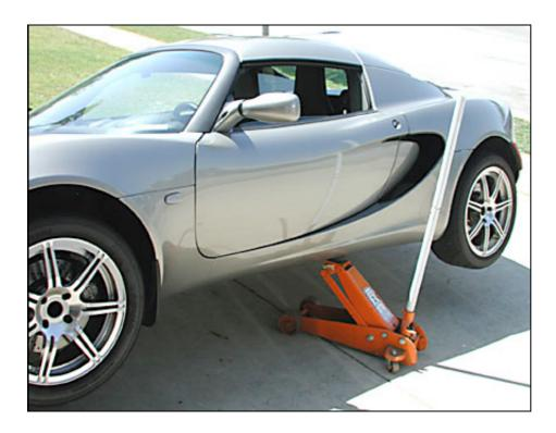
I do not recommend using just a jack to lift the car in order to complete the oil change. It is possible to remove the access panel, drain the oil, and remove the filter while the car is on a single jack. However I believe this is dangerous because the car is not stable and can fall off the jack or the jack can collapse.
