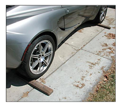
Block both the front and rear wheels on the opposite side of the car that you are going to jack up first. You can use any piece of wood or other stable material that will not roll. Slide the wood up against the tire.
