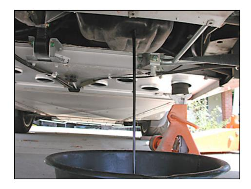
Remove the oil drain plug and take your hand out of the way quickly as the oil starts to pour out. Do not worry if you drop the plug in the pan, every one does it. Do worry if you see or hear bits of metal falling from the car into the drain pan as this is usually an indication of something broken inside the engine. This is not likely as the Toyota power plant has proven to be very reliable.
