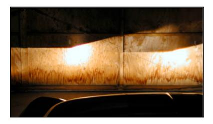
The Elise pattern shows a horizontal level cutoff to the left and a flair up and to the right. This provides illumination to the right side of the road. The bright spots in the center are not the high beam illumination pattern but are an artifact of the photography.
