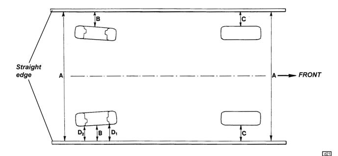
Measure the distance from the bar to the rim of the wheel concerned at the front and rear of the centre line of the wheel ( $D_1$ ,  $D_2$ ). If the front dimension,  $D_1$ , is greater than the rear dimension,  $D_2$ , the wheel has TOE-IN. If the rear dimension is greater than the front dimension, the wheel has TOE-OUT. The difference between the two measurements is the amount the wheel has toe-in or toe-out.
