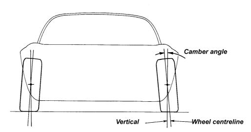
The primary purpose of camber is to achieve the maximum efficiency of the tyre under cornering loads and body roll, with the specification closely allied to a particular wheel/tyre combination. The camber angle changes with suspension travel, becoming more negative on bump, and should be measured only at the specified ride height. Incorrect camber can result in handling deficiencies and excessive tyre wear.
