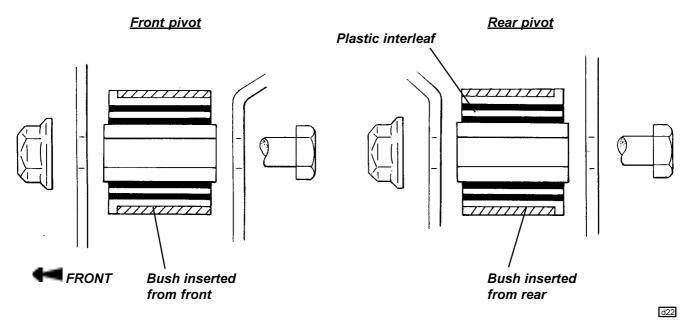
Lower wishbone rear pivot - insert a single 30mm long bush from the front end of the eye. Lower wishbone front pivot - insert a 16mm long bush into each end of the front eye.
