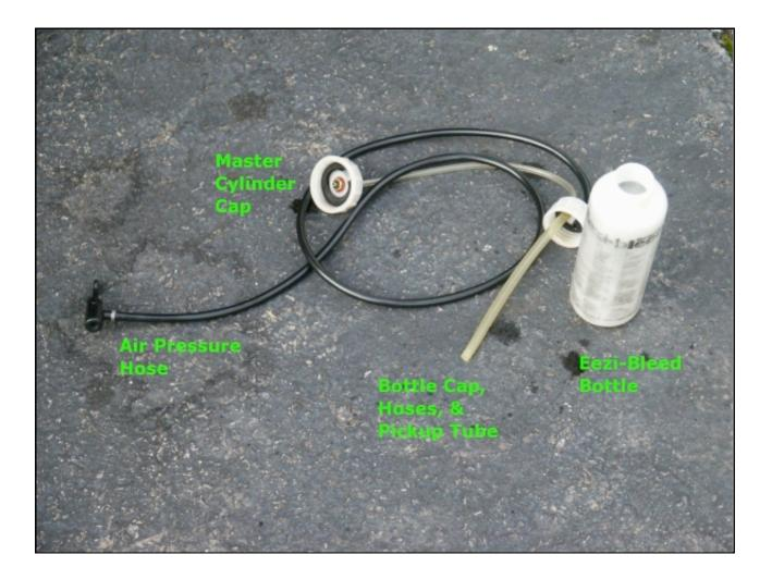
I have a "tool" that I made that has a tire valve fitting on one side, and an air hose coupler on the other. But this time, I used my portable air tank. The air tank is pressurized via a tire valve fitting - I added air until I had between 10-15 PSI on the pressure gauge. That's all the air pressure that you need to bleed the brakes.
